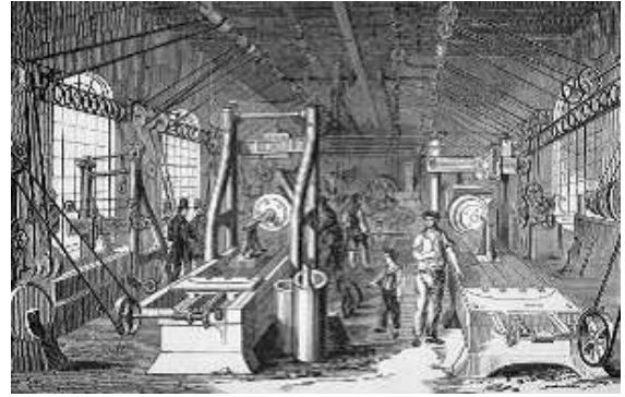
Fig. 6 – A fitting shop at a railway works in England, The Illustrated London News, 1849. In the fitting shop new locomotive engines were completed and old ones repaired.
