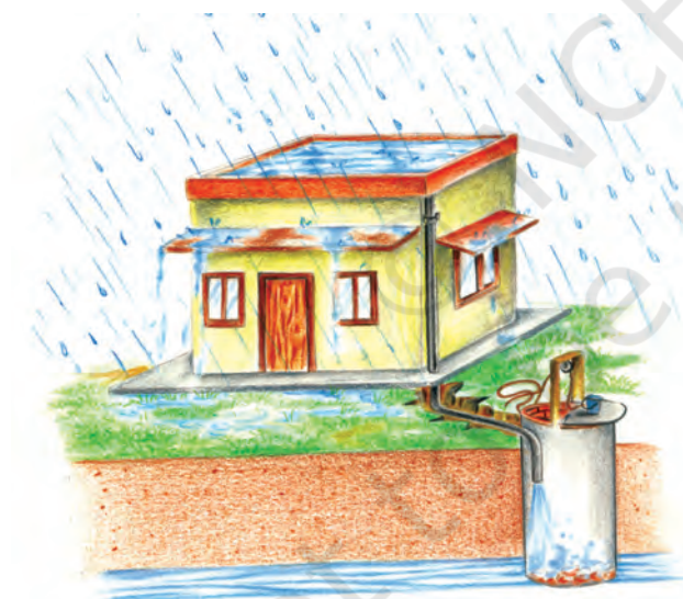
(b) Recharge through Abandoned Dugwell
